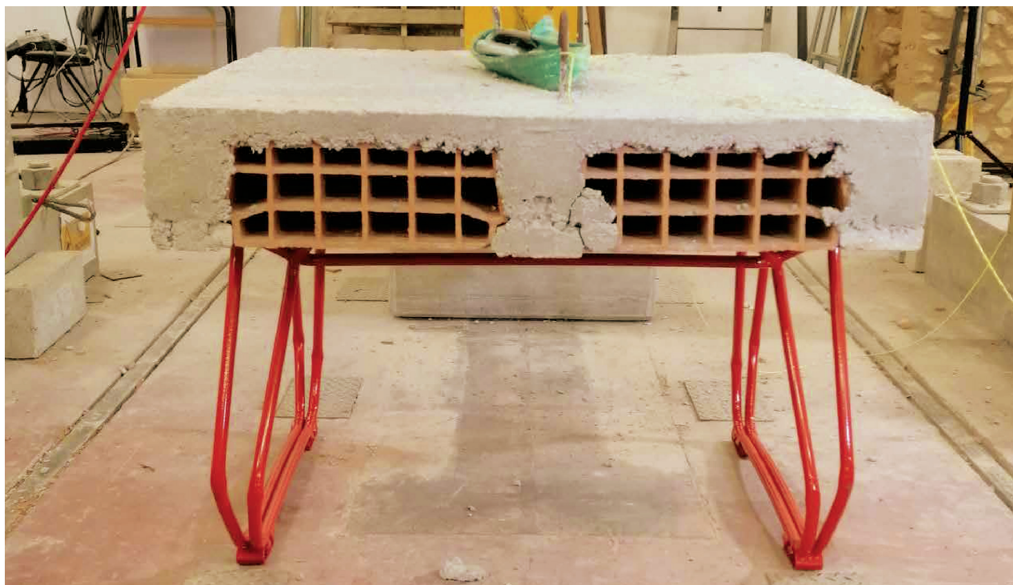
↑ Structural tests are being carried out to verify prototypes' resistance to the impact of falling rubbles
